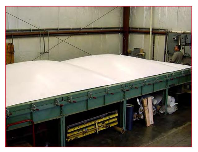
Simulated Wind Uplift Test - The stronger the seam, the greater the uplift resistance.
