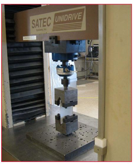
Breaking Strength Test DICP
