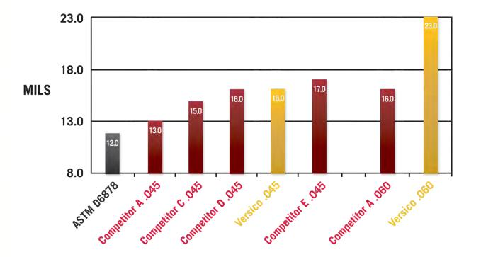
While it's important to have a thick sheet, which is measured in the "Thickness Overall" test, "Thickness Over Scrim" measures the top-ply of the TPO membrane. TPO consists of a top-ply, scrim in the middle and a bottom ply. The top-ply is the front line of defense against the elements and the usable life of the membrane is compromised when the scrim is exposed. Thickness over scrim is a critical measurement when evaluating the potential longevity of a TPO roofing system.
