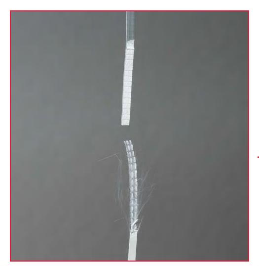
Desired Mode of Failure During Seam Peel Strength Test – Ply-to-Ply Separation
